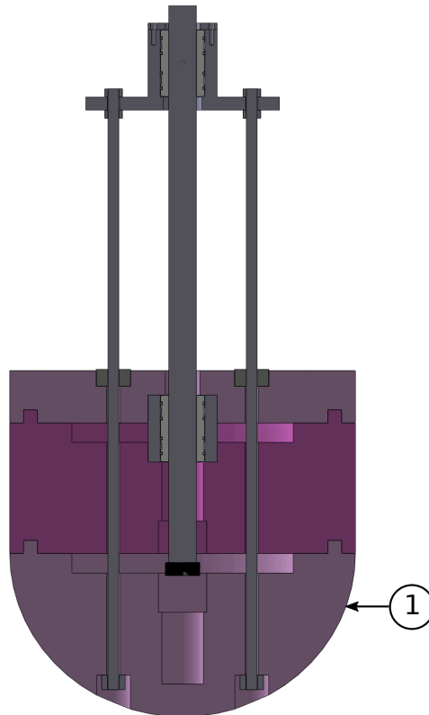
Figure 6.1: Physical model for the domed cylinder. The internal layout is identical to the truncated base so that the arrangement with the load cell for the fixed-body experiments is identical to that depicted in Figure 4.2. Key: 1. Hemispherical base
