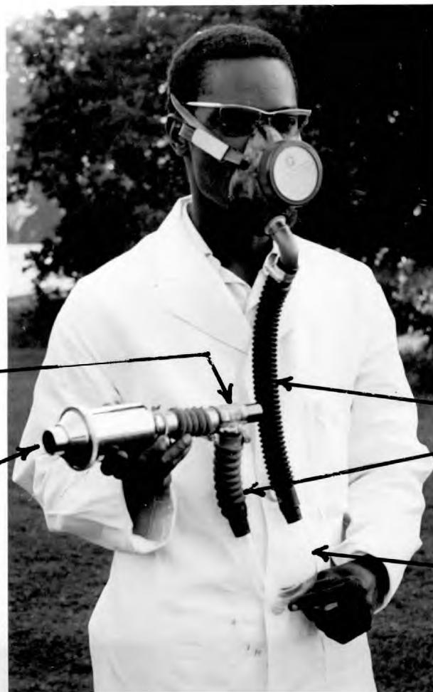
Fig. 30. Apparatus for the extraction of carbon dioxide from exhalent breath.
