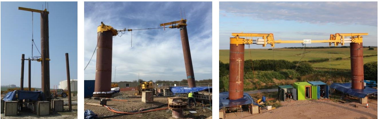
Figure 10: Images of the small ( D = 0.273 m), medium ( D = 0.762 m) and large ( D = 2.0 m) diameter test arrangements.
