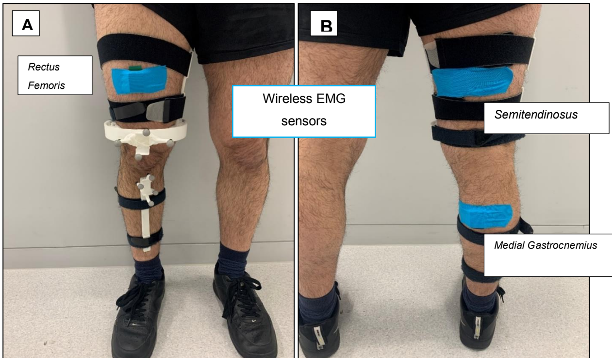
Figure 24: EMG placement secured by K-Tape with Assessment Rig in Situ
