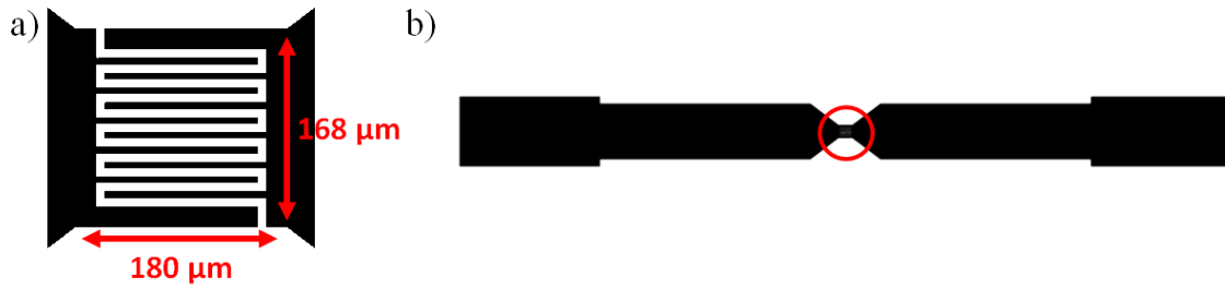
Figure 6.5: a) Geometry of the large comb (LC). b) Geometry of the short interconnects (SI).
