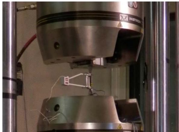
Figure 3. Coupon in INSTRON tensile testing machine.
