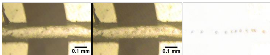
Fig. 14: The background composite image of a cell passage (left), the median composite image of the same cell passage (middle), and the resulting image of the cell only (right).
