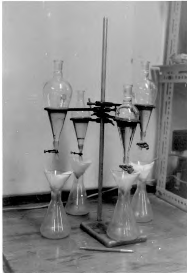
Figure 16. Apparatus used for heavy mineral separation.
