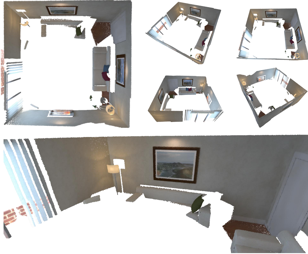
Figure 3.1: Tightly integrating IMU measurements into a dense RGB-D SLAM system leads to more accurate and robust tracking and 3D reconstruction compared with using visual information alone. For example, the scene reconstructed above has several large regions that lack photometric and geometric variation; despite this, the visual-inertial system described in this chapter was able to create a globally consistent reconstruction with flat and aligned walls.
