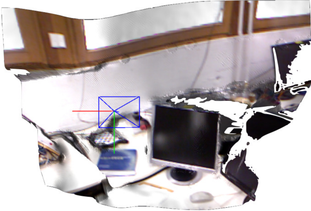
Figure 5.1: Fusing a single-view nonparametric depth probability distribution predicted by a DNN with standard photometric error terms helps to resolve ambiguities in the photometric error due to occlusions or lack of texture. The above projected keyframe depth map was created by the system. Despite a lack of photometric texture on the desk, walls and computer monitor, the system is able to create an accurate 3D reconstruction through the use of the data-based priors.
