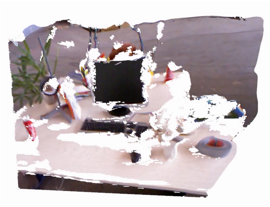
Figure 4.1: Fusing the depth predictions of a semi-dense multi-view stereo system with the depth and gradient predictions of a CNN allows for the creation of fully dense depth maps at scale. The above projected keyframe depth map was created by DeepFusion from only pose estimates and RGB images. Despite a lack of photometric texture on major scene components (such as the monitor and desk), which makes it difficult to obtain good multi-view stereo depth estimates, the use of learned priors allows for an accurate, dense 3D reconstruction.
