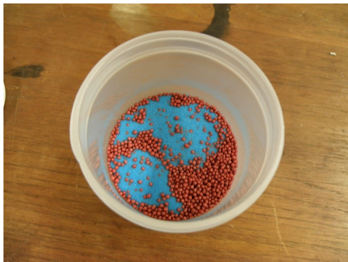
Figure 132. Aerial view of the small-medium filler sample after mixing. The two phases were unable to disperse throughout, due to the fineness of the sand.
