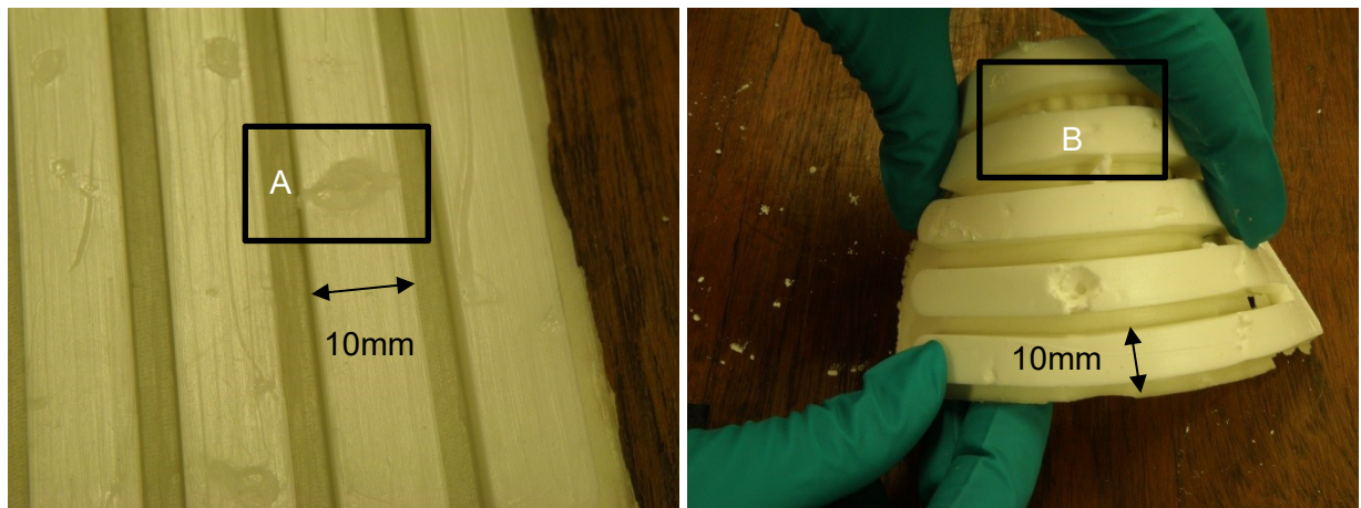
Figure 50. The 0.66 solid loading HTPB-DOS-Melamine-Barium Sulphate sample with visible indicators of inhomogeneity. Feature A is a pocket of uncured binder and feature B is a collection of powder agglomerations between the fingers of the sample
