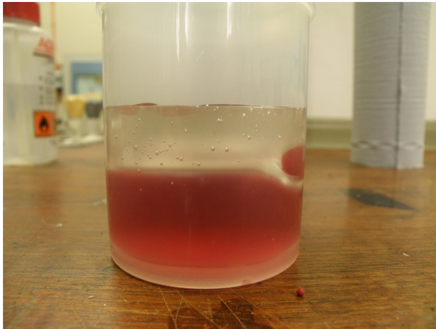
Figure 133. The liquid mixing experiment sample. Two different liquids were used; high viscosity HTPB and low viscosity water based sucrose solution. The water based sucrose solution was added after the HTPB but sunk through the HTPB to the bottom of the vessel
