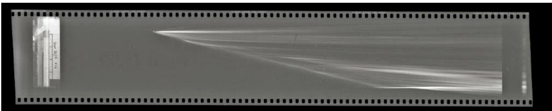
Figure 116. Streak camera film of Shot 2875 (LR 2). A static image of the sample is observed on the left hand side. As the mirror rotates within the streak camera at 6 \text{ mm } \mu\text{s}^{-1} the light from the sample detonation is projected onto the film. The VoD is calculated from the hypotenuse of the light using the known mirror speed and the length of the sample. Shot 2875 had a sample length of 19.6 cm
