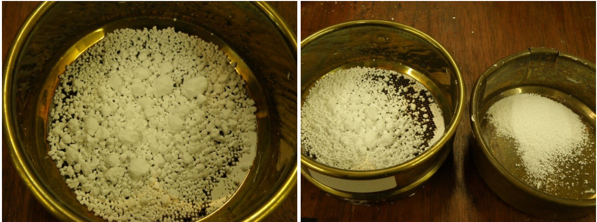
Figure 51. Pictured is the barium sulphate in a sieve with 1mm mesh size, comparing the powder that was used in the initial experiments and the powder that was used in the remaining experiments.
