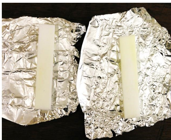
Figure 34. Modified image of LabRAM 0.80 solid loading DMA samples demonstrating colour variation. The yellowing colour is due to the oxidation of HTPB, and the inconsistent colour demonstrates an inhomogeneous sample
