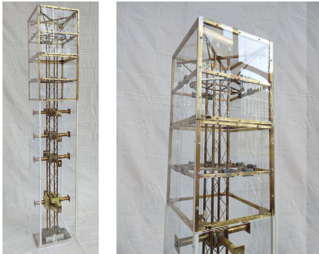
FIGURE 4 | Scaled physical model with rigid bars joining the skin and the core.
