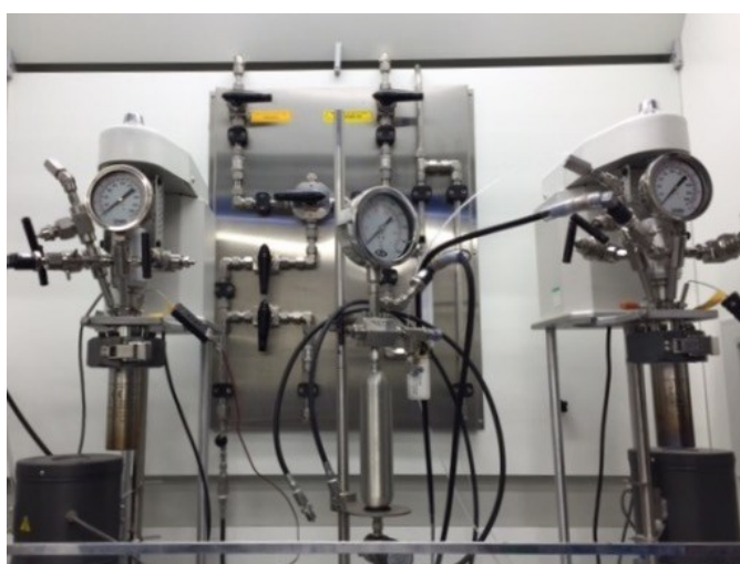
Figure 4.2.1 Parr Hastelloy autoclaves and gas control panel
