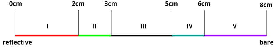
Figure 7.6: Geometry and boundary conditions for the one dimensional Reed cell radiation shielding benchmark test case.
