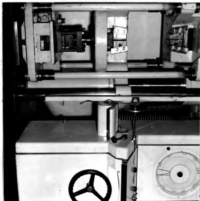
FIG.20 - COMPRESSION TESTING MACHINE AND SUBPRESS
