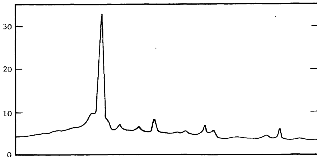
FIGURE 2.10: Gas chromatography analysis of impure sample of Ethoquad 18/25
