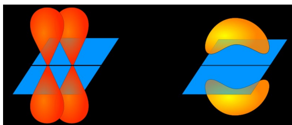
Figure 2.3: A delocalised \pi -bond above and below the molecular plane is formed by two p -orbitals.
