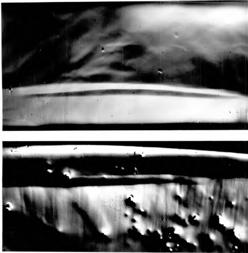
Fig 47. A kink along the tension edge of a beam of MgO deformed at 1500°C at a strain rate of approximately 5 \times 10^{-5} /min. The slip in the kink is in the 2D mode: Upper, from the tension surface, and lower from the side. x 40.
