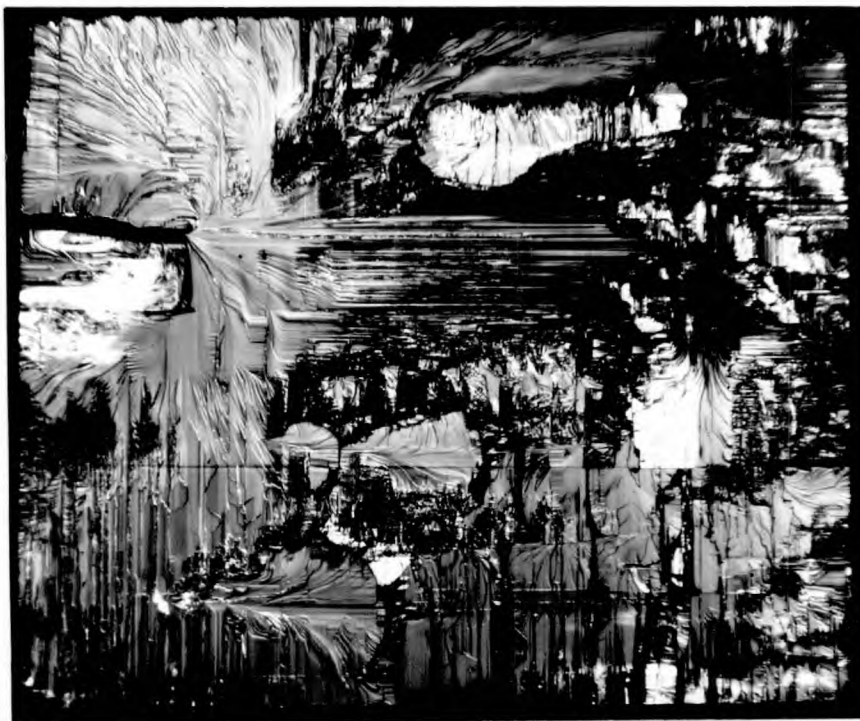
Fig 25. Complex fracture originating from a (101) slit. x 85.
