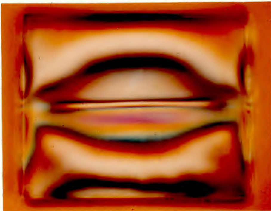
Fig 56. The same view as Fig. 55, but with \frac{1}{4} wave plates added to the optical system in a "mixed" orientation. \times 45 .
