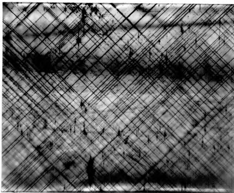
Fig 14. The expansion of many randomly orientated dislocation loops in MgO. x45.
