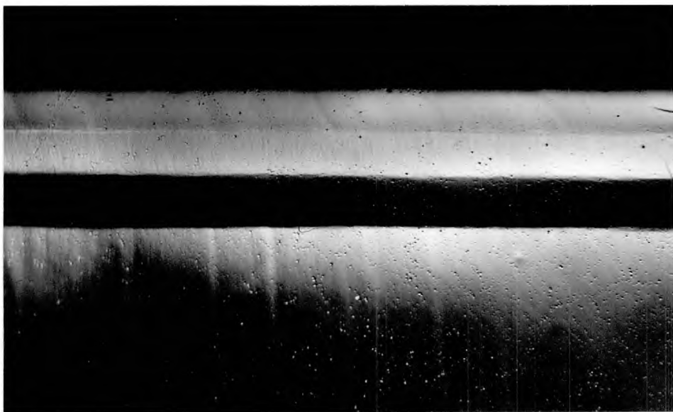
Fig 46. A double kink in a beam of MgO deformed at 1500^{\circ}\text{C} at a strain rate of approximately 10^{-5}/\text{min} . The slip in the kinks is in the 3D mode. \times 200 . (The tension surface)
