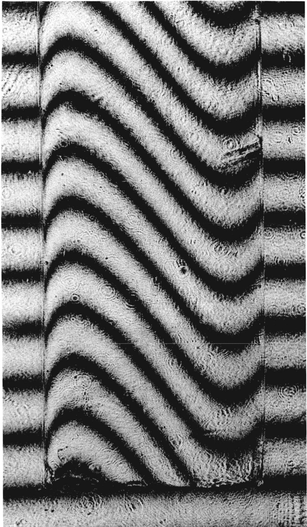
Figure 6.4: Experimental interferogram : An imperfect index match and a shearing misalignment
