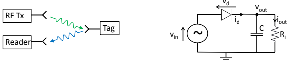
Fig. 1. System architecture (left) and single diode rectifier at the tag (right).
