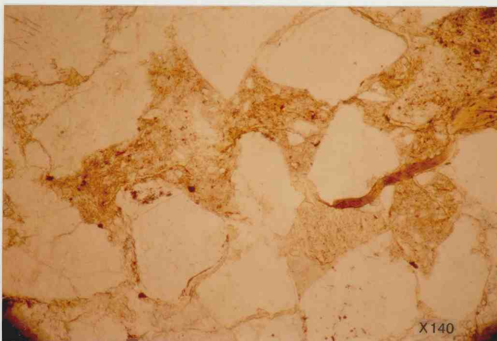
Fig.5.2. Photomicrograph of pseudomatrix resulting from plastic deformation and flowage of soft lithic grain. Plain light. Muladi-2 well. 4491m. Bhuban fm.
