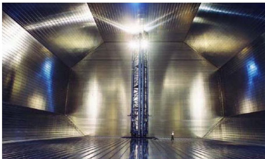
Figure 7.8: An illustration showing the inside features of a typical membrane tank LNG cargo containment system (GTT Website Illustrations).
