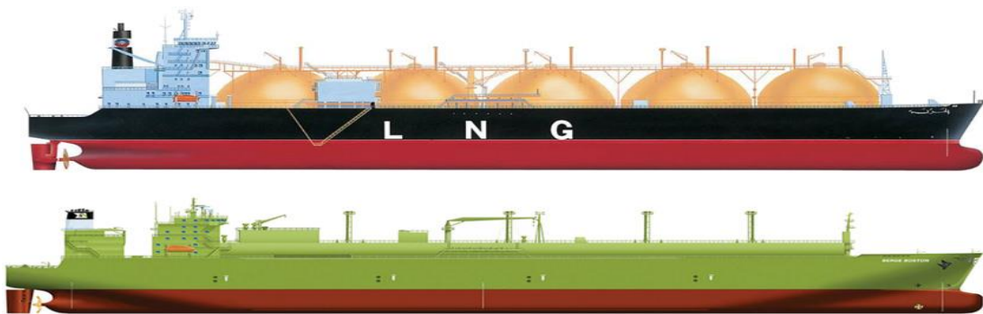
Figure 7.6: Features of a typical self-supporting spherical moss tanks (above) and the membrane type (below) (Vanem, 2008).
