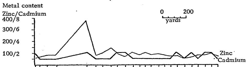
FIG. 11.11.5 CADMIUM, ZINC PRESENCE IN THE EDALE TRAVERSE
