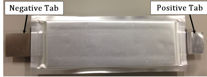
Figure 3.11: Kokam battery positive and negative tab
