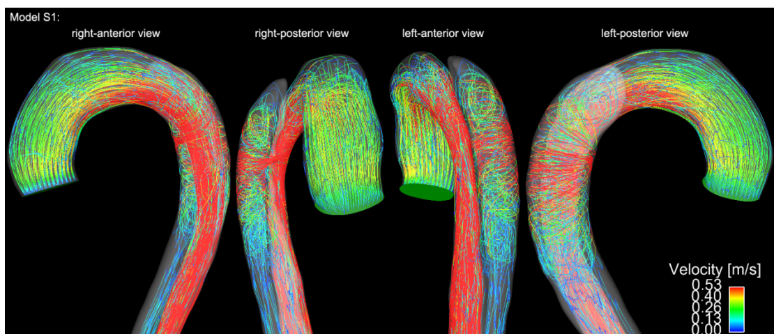
Figure 5.6: Particle paths of blood flow in aortic dissection model S1 from different view angles.
