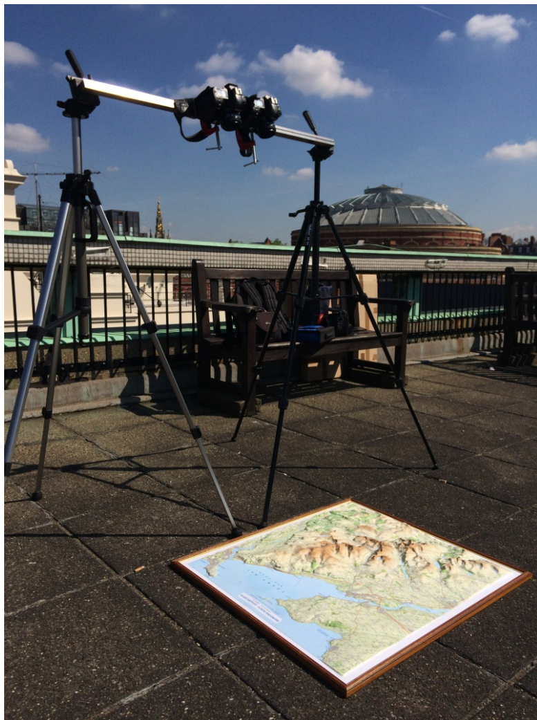
Figure 7.11 Stereo configuration to take terrain images under real sun illumination.
