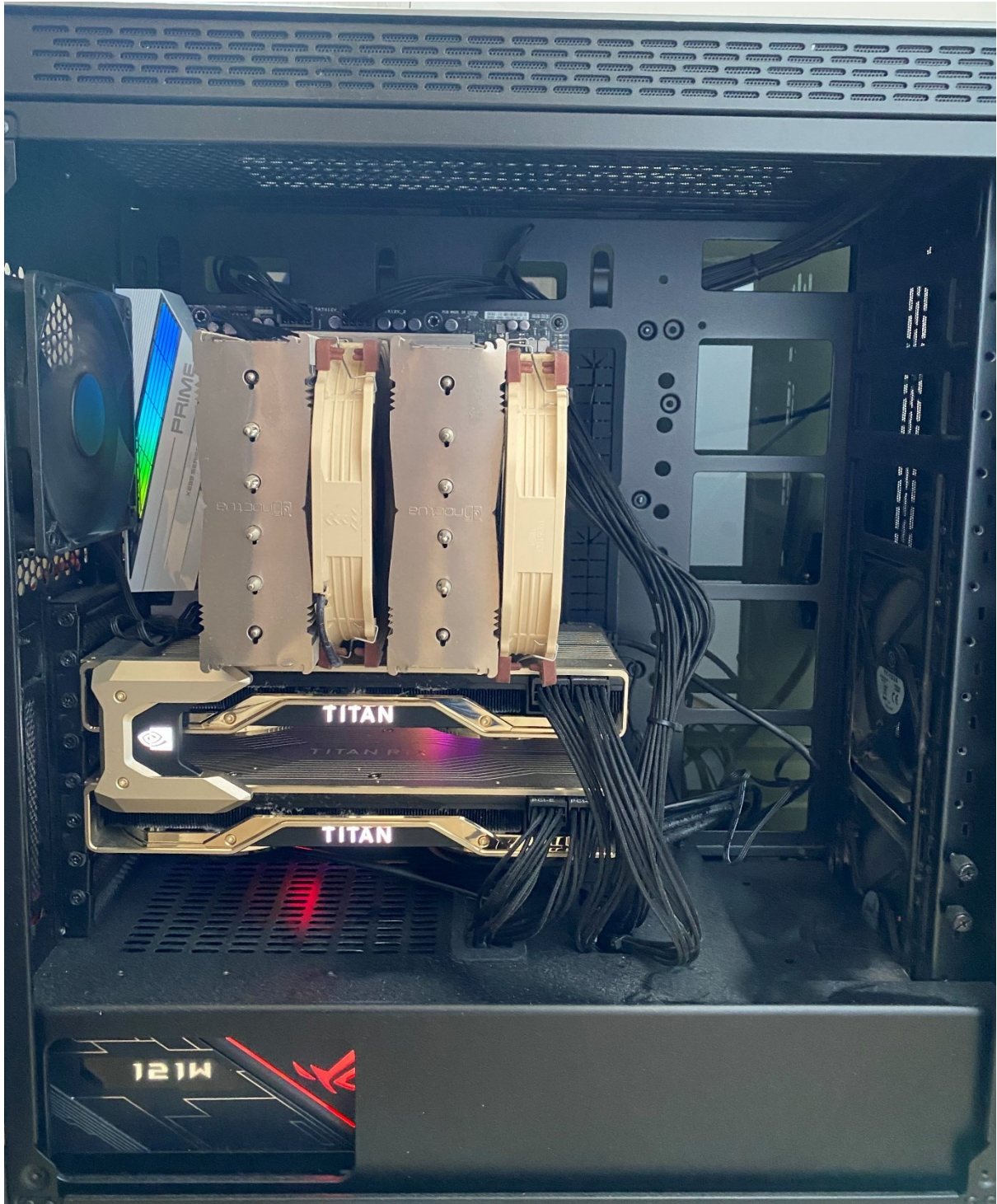
Figure 3-4 - The workstation used by the Student. Two RTX Titan graphical processing units (GPUs) are visible below the large central processing unit (CPU) cooler. The power supply at the bottom of the case shows the current power draw for the system in Watts.
