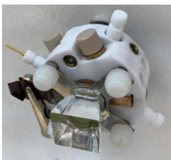
Figure 2. (A) Photograph of the CCPC-integrated PEC reactor. (B) Ray-tracing diagrams of a CCPC optic at selected angles between 0^\circ and 50^\circ , reproduced under the terms of the Creative Commons CC-BY 4.0 licence. Copyright 2023, X. Li et al. [15]
