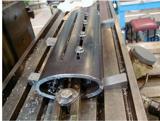
Figure 3. Machining of tensile coupons
