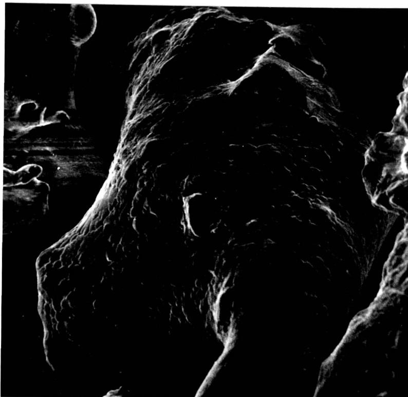
Stainless steel powder. Magnification X 1800
