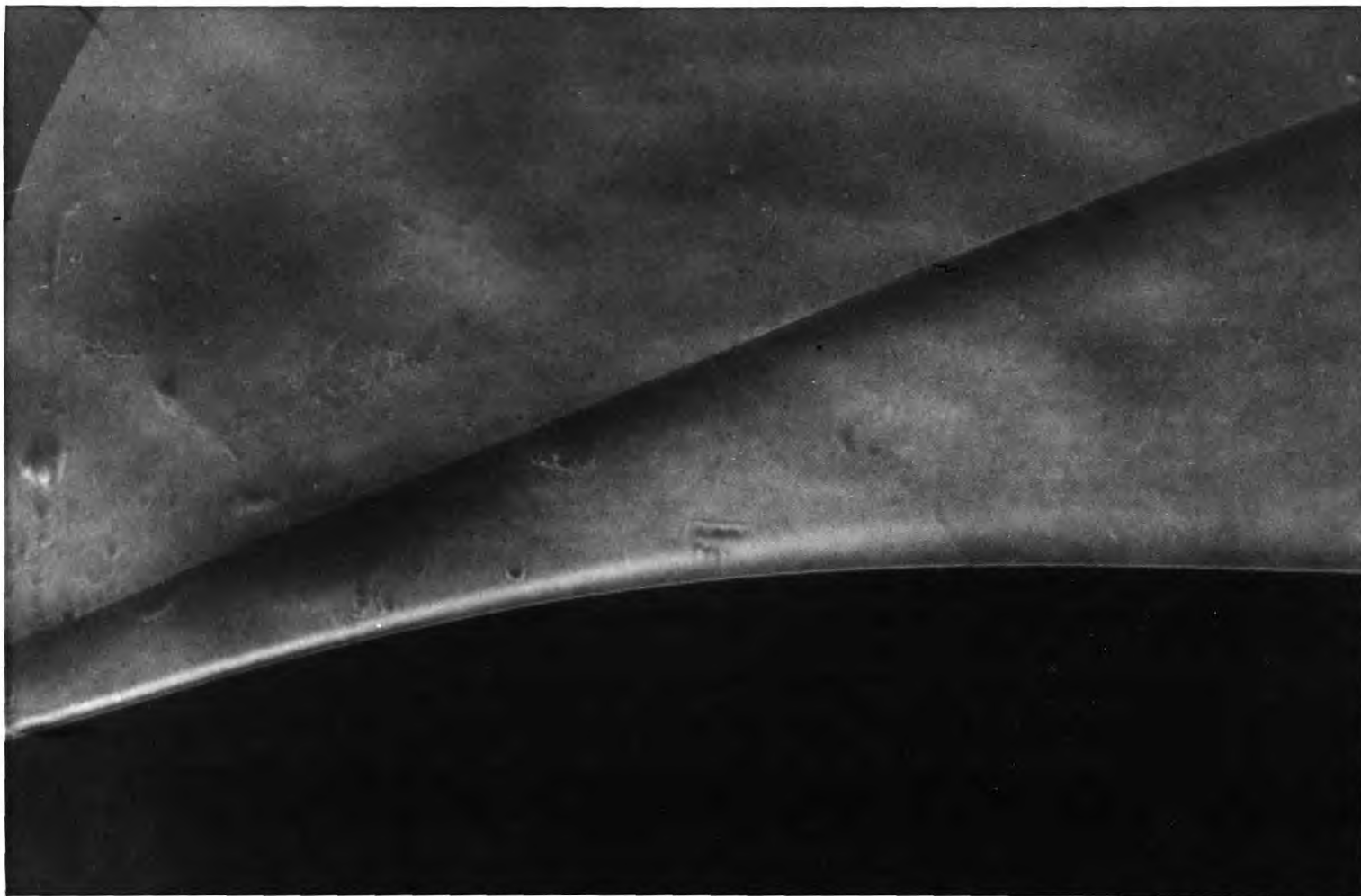
Fig. (16) Schlieren photograph of flow over the rear part of the convex surface. M = 12.25 , Re/\text{in} = 0.86 \times 10^5
