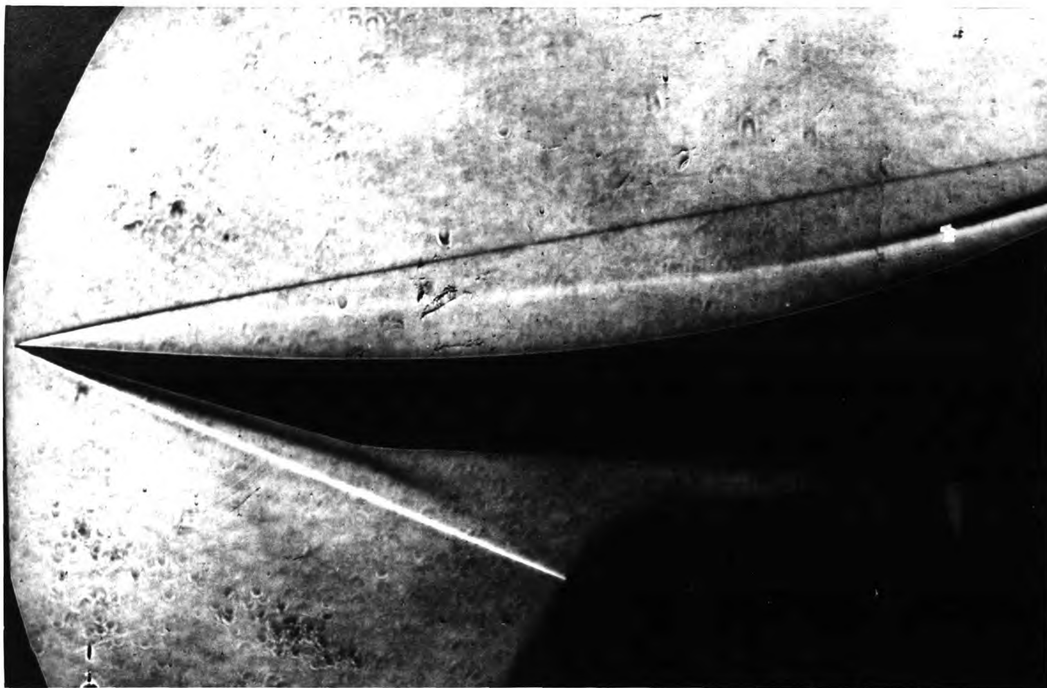
Fig. (14) Schlieren photograph of flow over cubic surface.
