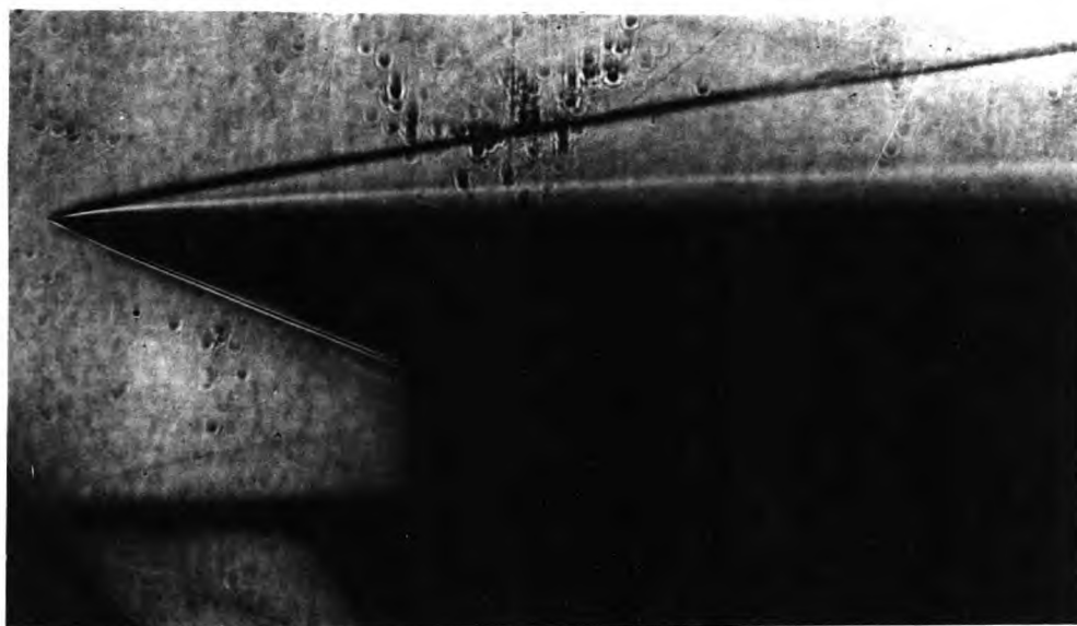
Fig.(6) Schlieren photograph of flow with a wedge model in the testsection
