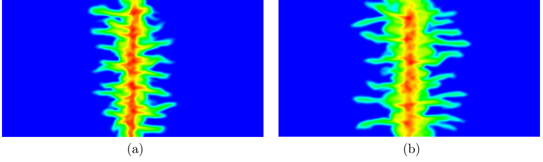
Figure 6.5: XZ density slices at stagnation. (a) LTE: 640 ns. (b) NLTE: 644 ns.
