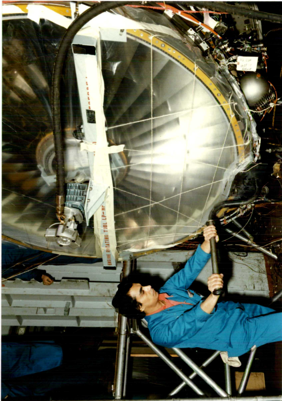
Figure 7.13 HP and IP Turbine Radial Probe Rotational Checks.
