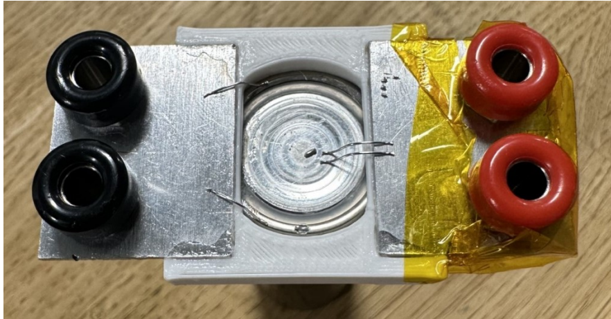
Figure 27 - Top view of a wire bonded cell before being placed in the test rig. Recreated from Ref. 180
