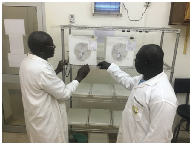
FIG. 2. Checking containment measures of the ACL 2 insectary facility at the IRSS Bobo-Dioulasso in Burkina Faso. Adult mosquito cages with rearing and maintenance record cards attached. A UV light device is hanging on the wall whose function is to catch free flying mosquitoes outside the primary barrier of a cage. Mosquito larval trays for breeding mosquitoes are covered with two layers of net to avoid escapes (Target Malaria © All rights reserved). Pictured: (left to right) Sougrinoma Zoungana (Senior Insectary Technician) and Charles Guissou (Senior Project Manager for Target Malaria Burkina Faso). UV, ultraviolet; ACL 2, Arthropod Containment Level 2. Color images are available online.
