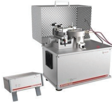
Figure 3.1: Anton Paar pin-on-disc test setup.
