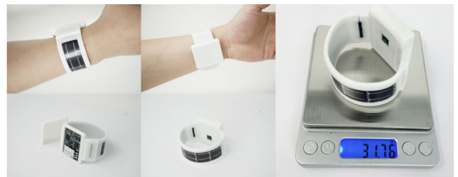
FIGURE 3. Overview of the solar-powered wristband prototype, weighed on an electronic scale with a total mass of 31.76 g.
