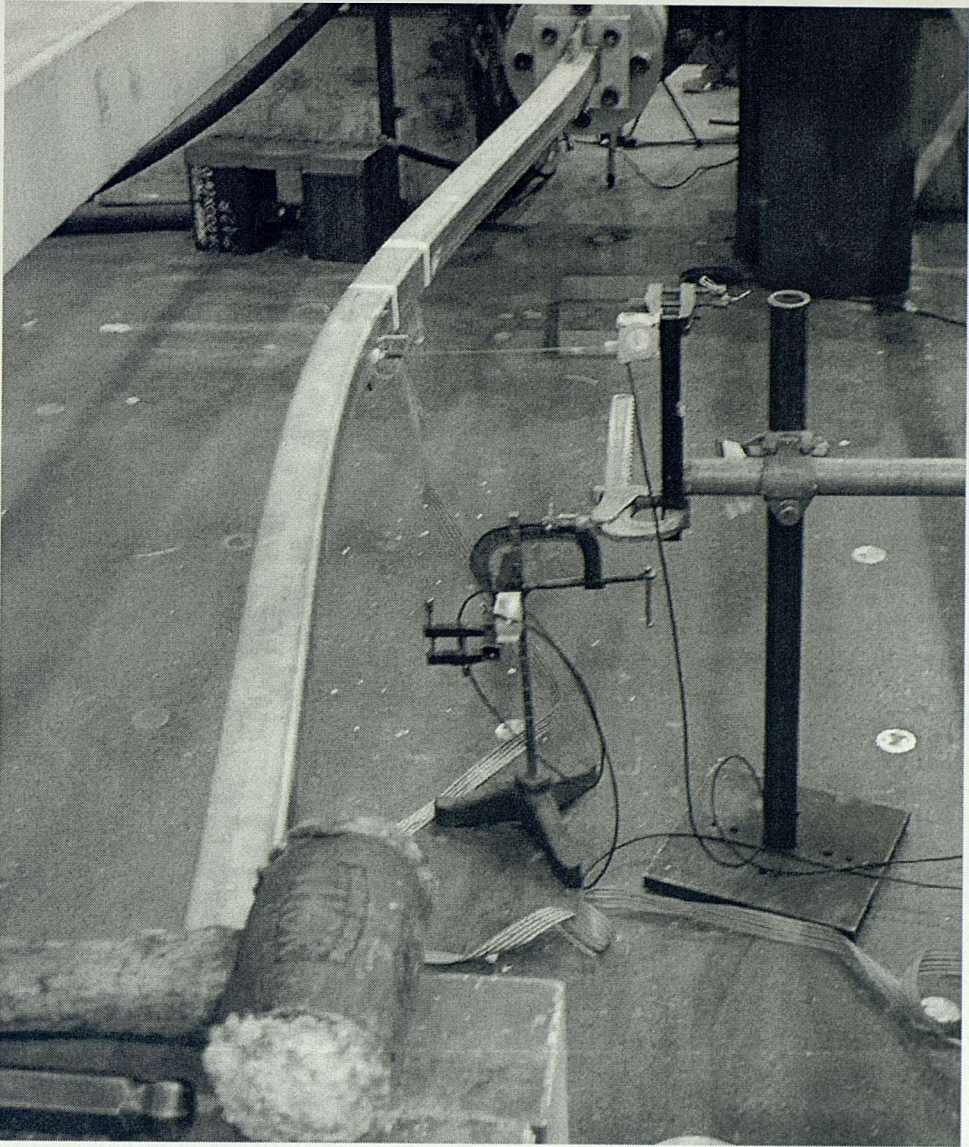
Figure 4.4: Buckling of specimen 60 \times 60 \times 3 \times 2850 -SS-CF
