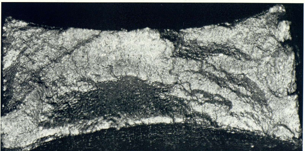
Figure 3.29: Mixed mode fracture surface shown on an axially loaded specimen tested at \pm 3\% strain amplitudes
