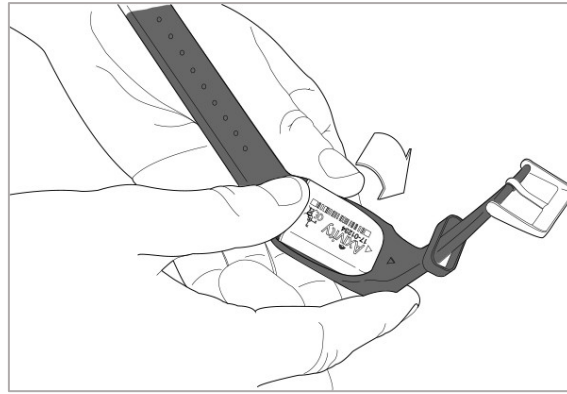
Figure 4.2. Sensor inserted into Axivity wrist band (Axivity User Guide: http://axivity.com/userguides/ax3/using/ )
