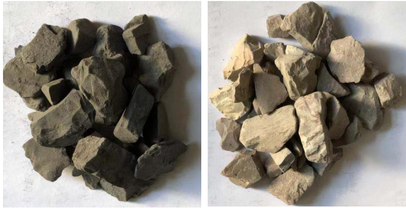
(a) Raw coal gangue (b) Calcined coal gangue
