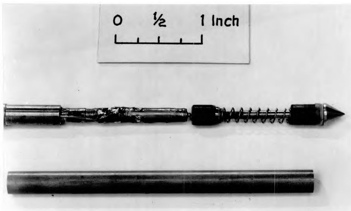
(b) Outer tube removed, showing base load cell and method of load application
