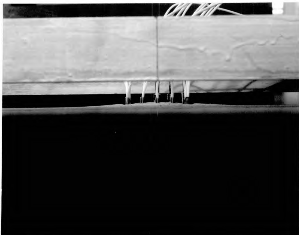
Heave of sand on driving 16 piles, spaced at 2d ; the sand surface of Plate 7.
