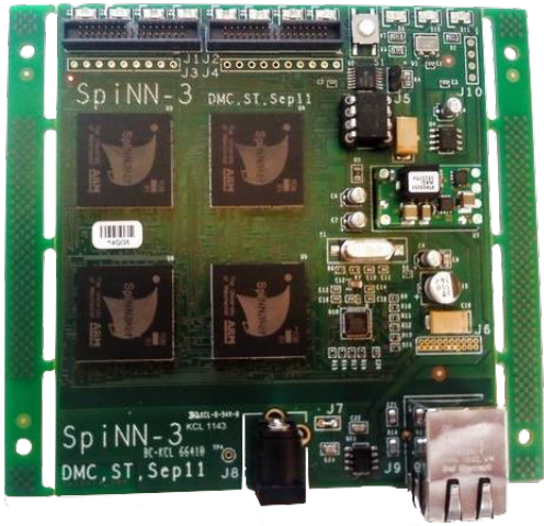
Fig. 1: The SpiNNaker I/O2 board use to prototype.
