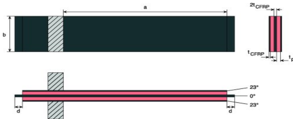
Figure 3. Schematic diagram of a polymer-interleaved composite beam specimen with different fibre orientations (36). (Black layers are composite laminae and red layers are polymer interleaves.)
