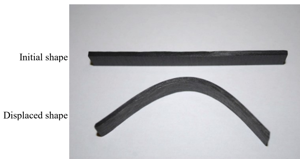
Figure 12. An image of the PS-interleaved flexure specimens in the initial and displaced shapes (125).
