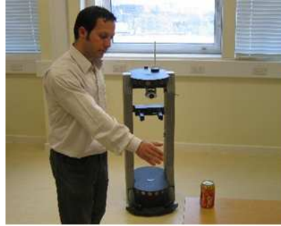
Figure 5: The experimental setup involves an ActivMedia Peoplebot observing a human demonstrator acting on objects
