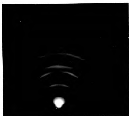
Fig.31. Silver deposited from K/4 silver nitrate solution in 10% water-dioxan mixture at 1 \text{ mA/cm}^2 and 20^\circ\text{C} . Weak (112) orientation.
