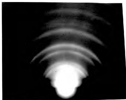
Fig. 40. Silver deposited under same conditions as for Fig. 38, but with \text{CS}_2 added to the bath.
