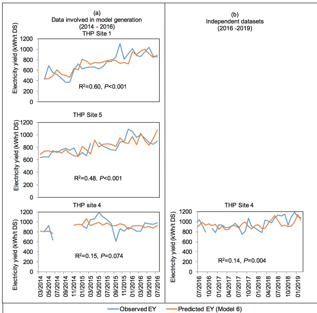
Figure 6-2 THP MAD model validation (Model 6) showing the time series of observed and predicted monthly average electricity yield for (a) THP Site 1, 5 and 4 for the data involved in model generation, and (b) THP Site 4 with independent data
