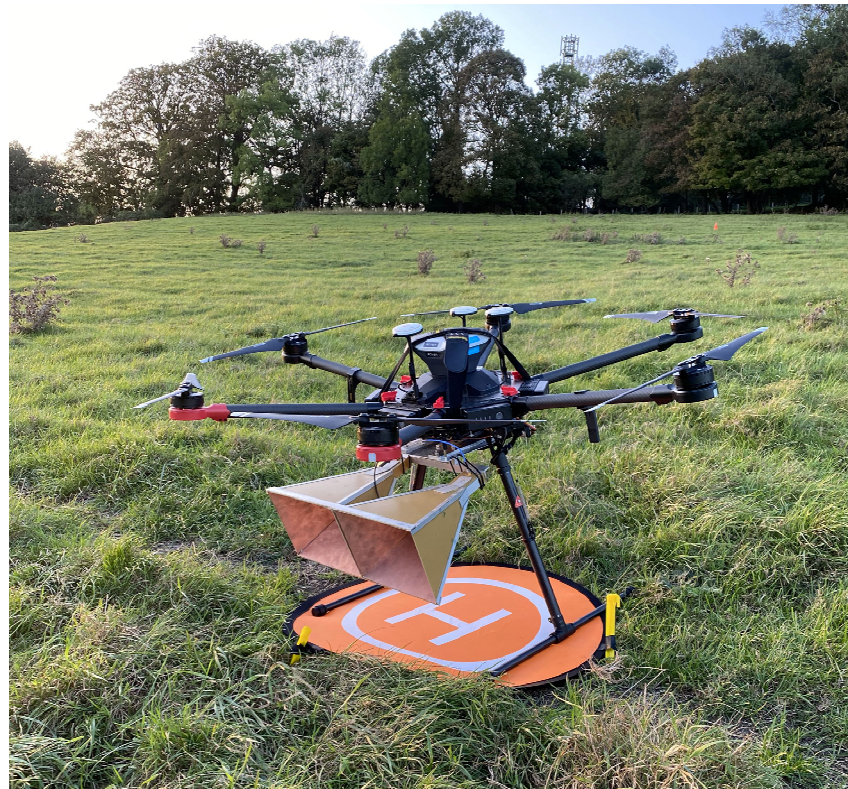
Figure 11. Drone radar payload attached to the drone at Flint Hall Farm.
