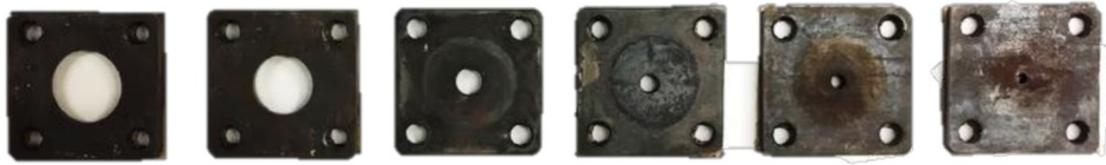
Figure 2.28 – Orifice Plates used for matching exercise; openings ranging from 1.5% to 100% of the exhaust pipe area
