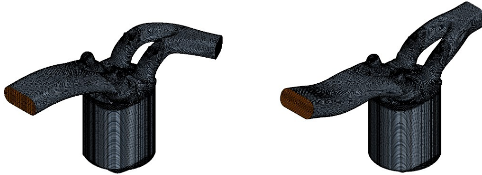
Figure 2.6 – Illustration of intake and exhaust ports design change between Build 1 and 2
