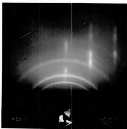
(b) Reflection pattern from solid Neon deposited at 7°K onto the (111) face of a silver single crystal. (The silver is not quite on azimuth.)
