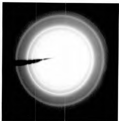
(b) Transmission pattern from Argon deposited at about 18°K.
