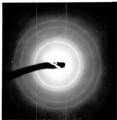
(a) Transmission pattern from solid Neon deposited at 7°K.
