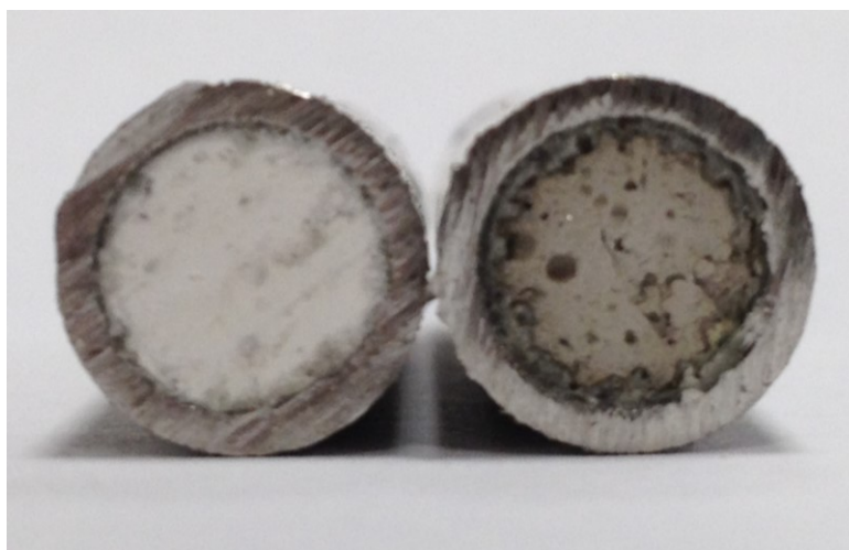
Figure 43. PolyHIPE within a flowcell before (left) and after (right) impregnation with palladium metal. Flow cell internal diameter 7 mm.
