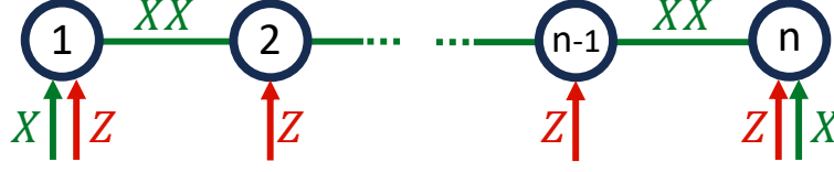
Figure 5.1: A linear spin chain of n qubits with nearest-neighbor XX interactions. Single-qubit Z -driving and X -driving on the end qubits facilitate the efficient preparation of various quantum states, such as GHZ and cluster states, and enable the realization of effective dynamics involving multi-qubit interactions.
